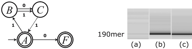
Fig. 4. (Left:) A 4-states automaton used for this experiment. (Right:) The results of electrophoresis are displayed in gel-like image. Lane (a) is for the input string 1101, lane (b) for 1110, and lane (c) for 1010. Since the full-length band (190 mer) is detected in lane (b) and (c), we determine the automaton accepts two input strings (b) 1110 and (c) 1010.
