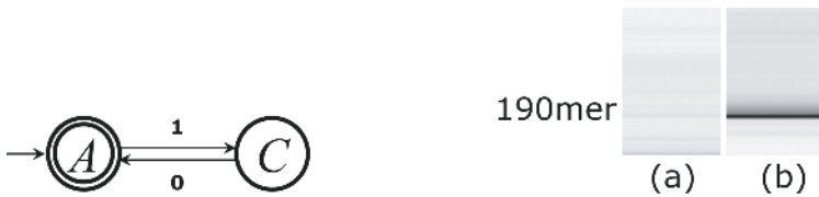
Fig. 2. (Left:) A simple 2-states automaton used for this experiment. (Right:) The results of electrophoresis are displayed in gel-like image. Lane (a) is for the input string 1101, and lane (b) for 1010. Since the full-length band (190 mer) is detected only in lane (b), we determine the automaton accepts only the input string (b) 1010.
