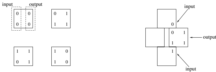
Fig. 1. The set of four tiles on the left implements the operation \oplus . A tile glues to other tiles only if their corner labels match. On the right, operation 0 \oplus 1 = 1 is performed. The input tiles are preassembled and the correct output tile simply attaches itself to the pattern, effectively obtaining the value of the output bit.
