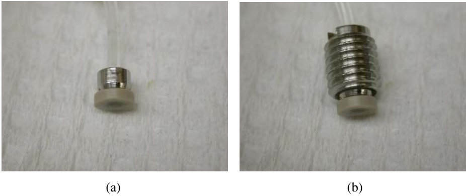
Fig. 1. (a) A ferrule with a frit. The plastic part of the ferrule has a filter, i.e. a frit, embedded in it. This can be used to retain beads in tube sections. (b) A nut falls over the ferrule. By tightening the nut, the metal part of the ferrule pushes down on the tube, effectively immobilising the tube.
