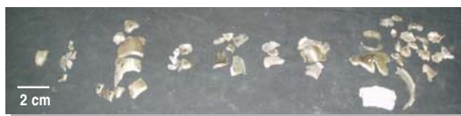
Fig. 4. Retrieved fragments from explosively driven AerMet 100 pipe
