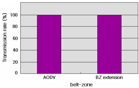
Fig. 16. Transmission success rate of AODV and that of extended BZ in low density
