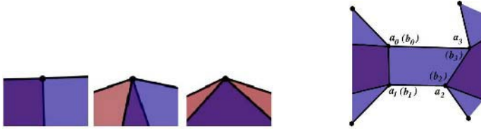
Fig. 5. (left 3 images) Frozen V-V ties (group A, pink; group B, blue; A \cap B , purple); (right image) Unwanted lock formed by frozen ties (Group A, purple; group B, blue)
