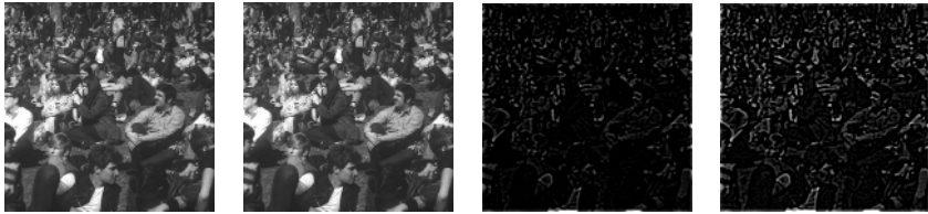
(a) crowd image (b) compressed image (c) bipolar cell output (d) amacrine cell output
