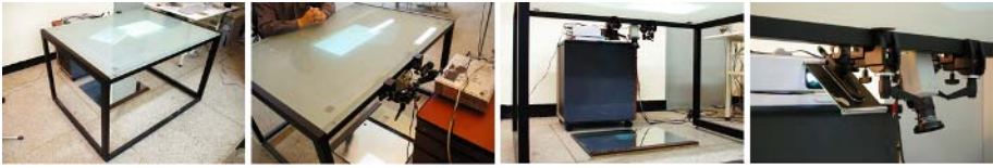
Fig. 2. Implementation: a frame, a projector, a camera, and mirrors
