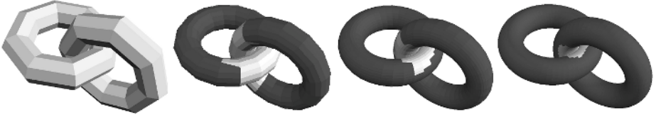
Fig. 4. The intersection algorithm proceeds from left to right, subdividing and updating the graph at each iteration. Faces still in the graph are highlighted. Note that most faces are excluded at a low resolution.
