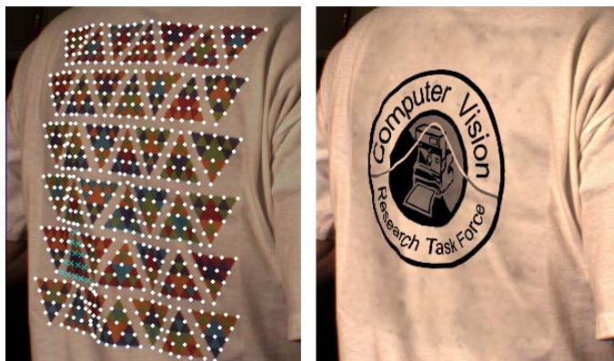
Fig. 6. Specialized patterns make it possible to track very large numbers of points. However, such large numbers are not necessary and can even be slightly detrimental: irradiance estimation becomes difficult because more pixels are classified as edge pixels. In comparison to Figure 2, the irradiance estimates here are visually less accurate.
