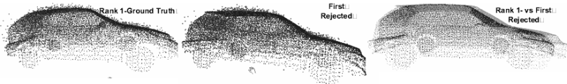
Fig. 7. Better coverage and less similarity between models result in only one identified model using saliency, compared to 15 models returned as possible candidates by the matcher. Query is Geo Metro 1990 plotted in red. Note the dissimilarity in the front between the Geo Metro 1990 (dark gray) and a Honda Civic 1990 (light gray) which is the rejected model ranked second using global scores (rightmost figure).
