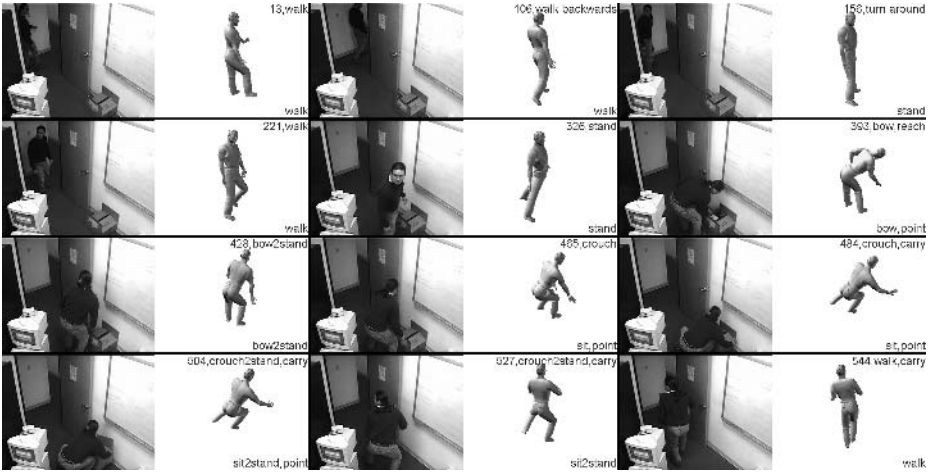
Fig. 3. Key frames of one annotated video. Ground truth and recognition result is shown in top-right and bottom-right, respectively.
