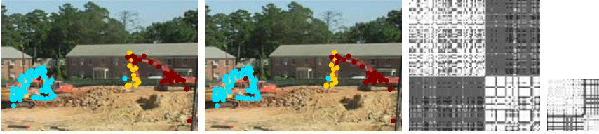
Fig. 5. (left 2) A sequence of two bulldozers moving independently, one of which moves articulately with its arm rotating around an axis. The color of a dot, red, blue or yellow, shows the segmentation result. There is one misclassification error which is the red dot on the forearm near the axis. Besides that, there are several outliers. (right 2) The affinity matrices for 2-stage segmentations are shown. The row and columns are rearranged based on the segmentation.
