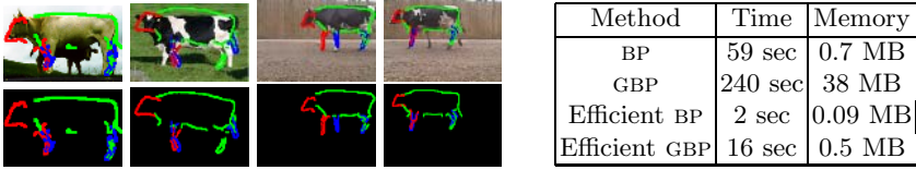
Fig. 4. Results of obtaining the MAP estimate of the parts of cows using the fast, memory-efficient GBP. The first row shows the input images. The detected parts are shown in the second row. The table on the right shows the average time and space requirements of various methods for object recognition.
