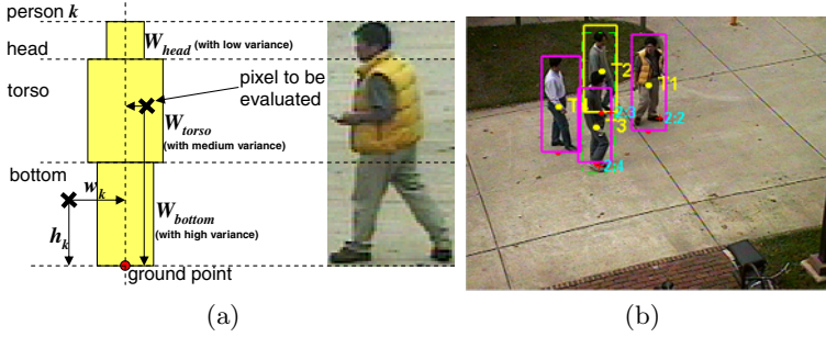
Fig. 1. (a) Illustration of appearance model, (b) Bounding box detection
