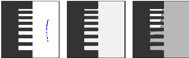
Fig. 1. Left: Initialization superimposed on the initial image; center: no viscosity, \nu = 0 ; right: \nu = 1.0
