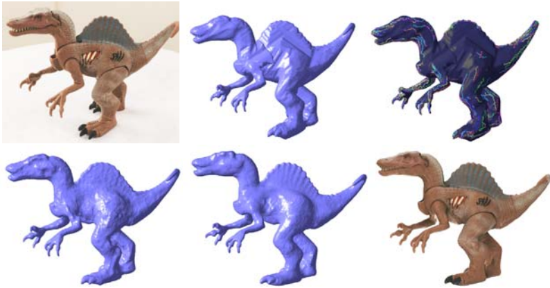
Fig. 1. Overall flow of the proposed approach. Top: one of the 24 input pictures of a toy dinosaur (left), the corresponding visual hull (center), and the rims identified in each strip using dynamic programming (right). Bottom: the carved visual hull after graph cuts (left) and iterative refinement (center); and a texture-mapped rendering of the final model (right). Note that the scales on the neck and below the fin, as well as the undulations of the fin, are recovered correctly, even though the variations in surface height there is well below 1mm for this object about 20cm wide.
