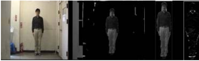
Fig. 12. Background subtraction method: (from left to right) original image, background subtracted image, segmented image and Sobel edge image
