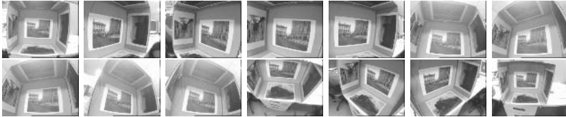
Fig. 3. Box dataset: photographs taken of a test rig (consisting of photographs pasted to the inside of a cuboid) with strong changes of perspective, changes in scale and large amounts of radial distortion. This tests the corner detectors on planar textures.
