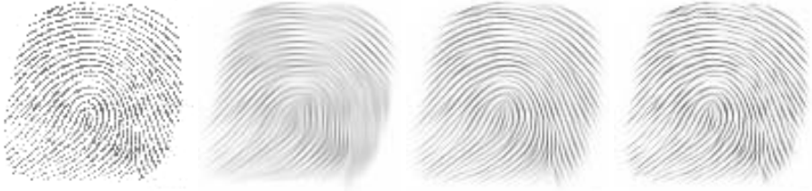
Fig. 5. Left to right: (a) Fingerprint image, 100 \times 100 pixels. (b) Filtered with the nonnegativity scheme [25] for CED with C = 1 , \sigma = 0.5 , \varrho = 4 , \tau = 1/6 , and N = 60 iterations. (c) Processed with our LSAS algorithm for CED, same parameters. (d) LSAS algorithm with \tau = 1 and N = 10 iterations.
