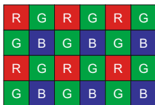
Fig. 1. The Bayer color filter array pattern
