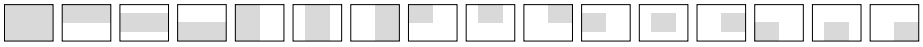
Fig. 2. Local sampling scheme for tentative motion models. Samples are drawn from sub-regions of the image plane to exploit spatial coherence and reduce the required sample number.
