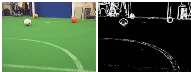
Fig. 7.16. Left: image of a RoboCup scene including the three kinds of balls that were used for training the classifier. Right: the corresponding edge image generated with a Sobel filter. The classifier was trained on such images
