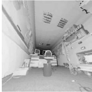
Fig. 7.11. Image of a chair with strong occlusion. In this example, a recognition with the Viola-Jones Classifier was not possible
