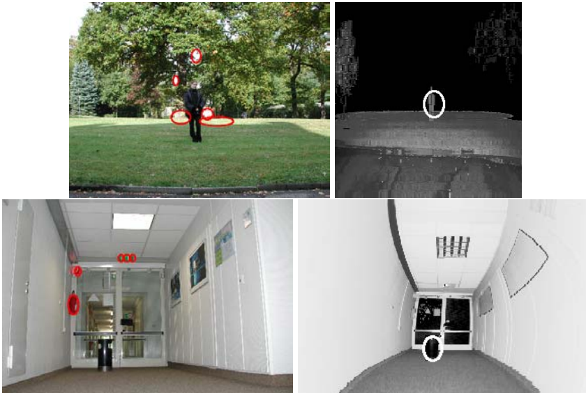
Fig. 6.14. The foci show some advantages of the laser data: the person (top) and the rubbish bin (bottom) are only focused in the laser data (right), but not in camera images (left). The bottom example shows the respective advantages of the sensors: the FOA in the laser data is on the rubbish bin whereas the FOAs in the camera image are on the fire extinguisher and the emergency exit sign
