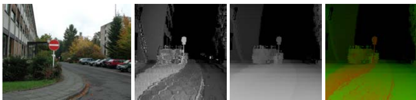
Fig. 6.3. Combining depth (2nd) and reflection (3rd) image into one colorized image (right). Range is coded as intensity, reflection as red-green transition
