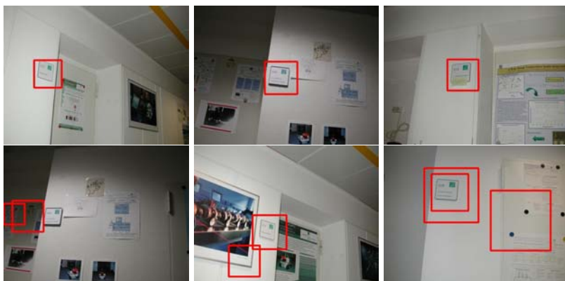
Fig. 7.14. Classifying name plates with the classifier of [Viola and Jones, 2004]. First row: perfect classification. Second row: one miss, 4 false detections and one double detection
