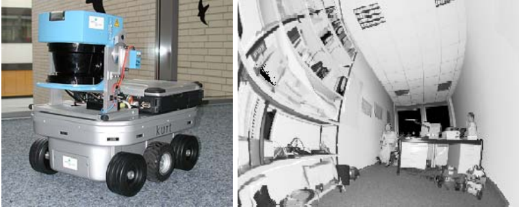
Fig. 6.1. Left: the custom 3D range finder mounted on top of the mobile robot Kurt3D. Right: an office scene imaged with the 3D scanner in reflection value mode, medium resolution ( 361 \times 211 pixels, distortions not corrected)
