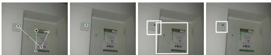
Fig. 7.15. Searching for name plates. From left to right: 1) The first 5 FOAs by pure bottom-up attention, the 5th FOA is on the name plate. 2) The 1st FOA by top-down attention searching for name plates. 3) A false detection found by the classifier while scanning the whole image. 4) No false detection occurs when concentrating on the first region of interest found by the attention module
