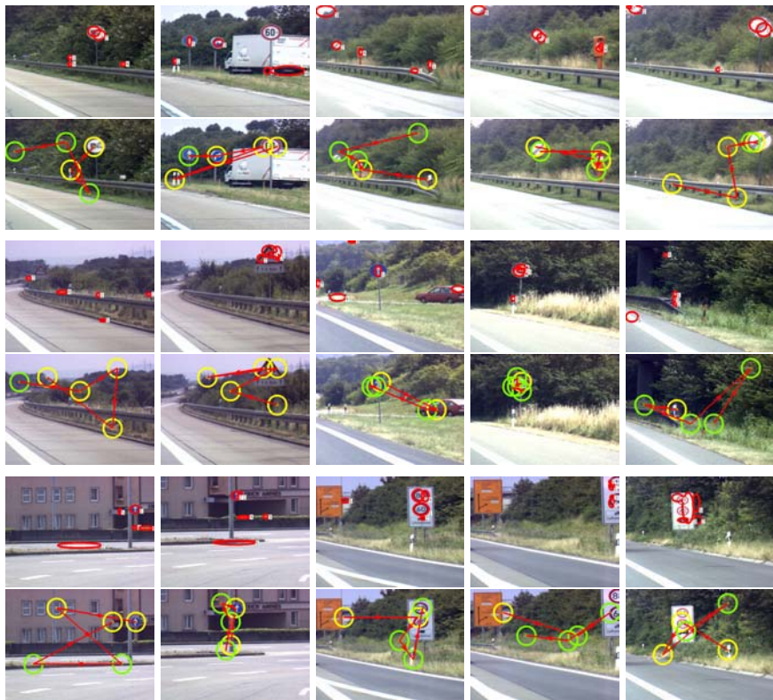
Fig. 4.23. Comparison of VOCUS with the NVT [Itti et al., 1998] on a test set of Laurent Itti ([URL, 07]). The FOAs of VOCUS are depicted as red ellipses, the FOAs of the NVT as yellow circles. On these images, an objective evaluation is not possible, they are just displayed to get an impression of the differences
