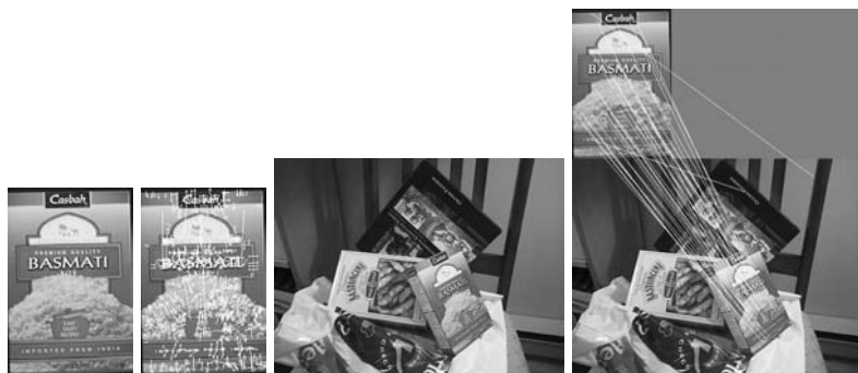
Fig. 7.7. Testing Lowe’s SIFT Keypoint Detector [Lowe, 2004, URL, 13] for a complex target (basmati rice box). From left to right: 1) Training image. 2) 572 keypoints on training image. 3) Test image. 4) Test image in which 38 keypoints match. For such complex target objects, the recognition is successful even if the target is presented from different viewpoints (original images from [URL, 13])
