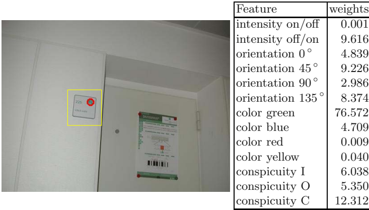
Fig. 5.3. Learning the target “name plate”. Left: a region of interest (ROI) detected by a classifier (yellow rectangle) and the most salient region (MSR) inside the rectangle (red ellipse). Right: the weights for 10 feature and 3 conspicuity maps learned from the MSR. The green color feature map has the highest weights value
