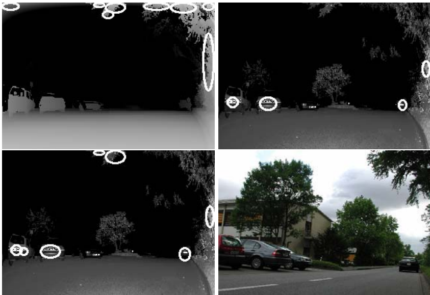
Fig. 6.11. The foci in laser data show some advantages of the reflection mode. In reading order: depth image, reflection image, combined image, camera image. All of the four cars are among the first six focus regions in the reflection data
