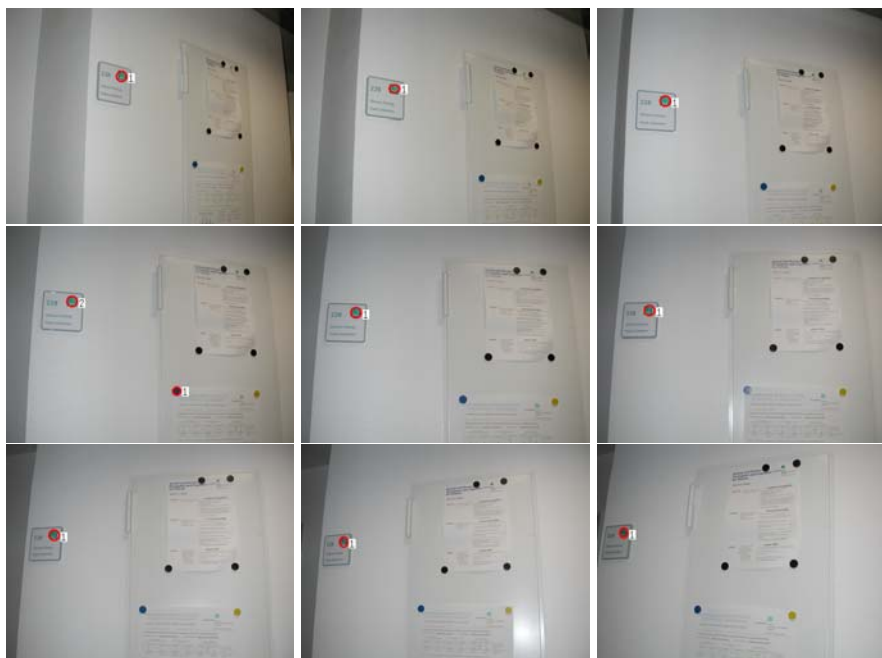
Fig. 5.16. Search for name plates under viewpoint changes. The same scene was regarded from 9 viewpoints, each about 40 cm distant from the next one. The hit number is always 1, only in one image it is 2 (middle row, left)
