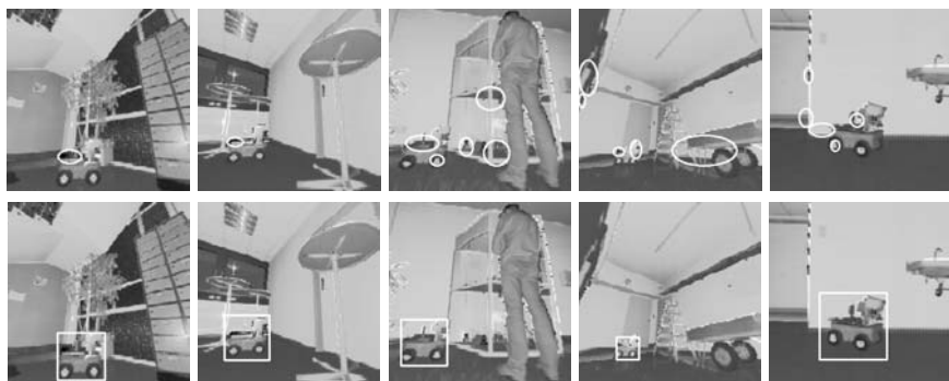
Fig. 7.13. Attentive classification in laser data. Top row: the first resp. the first 5 foci of attention computed on depth and reflection data. Bottom row: classified objects in the focus regions. Right: a robot rotated by 30^\circ is still detected
