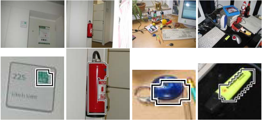
Fig. 5.13. Top: some training images with targets (name plate, fire extinguisher, key fob, and a highlighter on the dark desk). Bottom: The part of the image that was marked for learning (region of interest (ROI)) and the contour of the region that was extracted for learning (most salient region (MSR))
