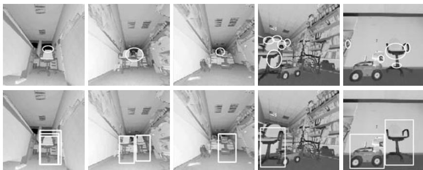
Fig. 7.12. Attentive classification in laser data. Top row: the first resp. the first 5 foci of attention computed on depth and reflection data. Bottom row: classified objects in the focus regions. Left to right: 1) Chair is detected even if the focus is at its border; 2) detection of two chairs; 3) chair is detected although it is presented sideways and partially occluded; 4) only the chair is focused, therefore the chair but not the robot is classified; 5) both objects are focused and classified
