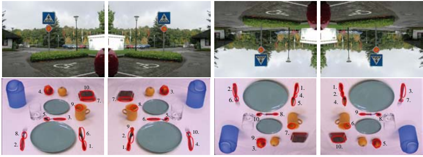
Fig. 4.24. Foci in flipped images. First row: the 1st focus on the traffic sign is stable because its saliency value differs clearly from the value of the 2nd focus. Second row: the first 10 FOAs on a breakfast table image. Similar saliency values result in slight changes of position and order of the FOAs
