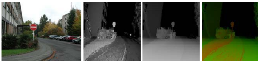
Fig. 6.3. Combining depth (2nd) and reflection (3rd) image into one colorized image (right). Range is coded as intensity, reflection as red-green transition
