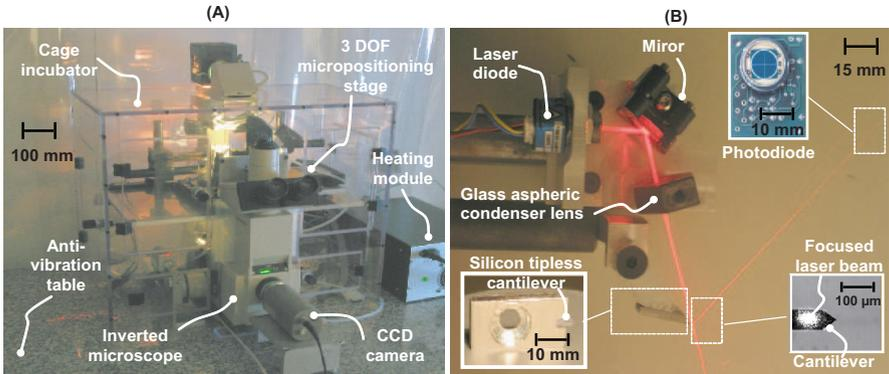
**Fig. 1.** (A) The *FBM* experimental setup overview. (B) The mechanical sensing unit.
