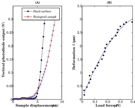
**Fig. 5.** (A) Experimental data of the photodiode output as function of the sample displacement performed on both single *EpH* cell and hard surface. (B) Experimental curve of the sample deformation  $\delta$  as function of the applied load by the cantilever.
