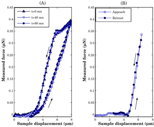
**Fig. 6.** (A) Experimental spectroscopy curves (approach and retract) performed on a single *EpH* cell at different time intervals ( $t=0$  mn, 40 mn and 80 mn). (B) Single referenced approach and retract curves performed on hard surface.
