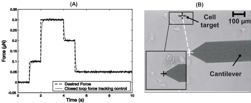
**Fig. 2.** (A) The force feedback control approach. (B) The vision feedback control approach.
