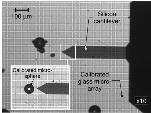
**Fig. 3.** Pixel to real world calibration of the CCD camera using the calibrated glass micro-array.
