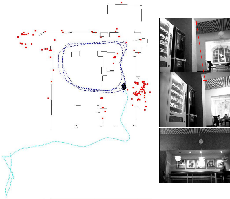
Fig. 5. The SLAM map is shown as red squares at the locations of landmarks. To help visualize the environment, a separately made laser scanner map is superimposed on this map. Also shown are the trajectories from when the map was built (3 loops) and when the robot was trying to localize. The feature match between the evening database image image (top) and the daytime localization experiment (middle) is indicated. The bottom image corresponds to the area of the map where the density of landmarks is greatest.
