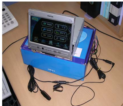
Fig. 5. Embedded system using an AutoPC for car navigation
