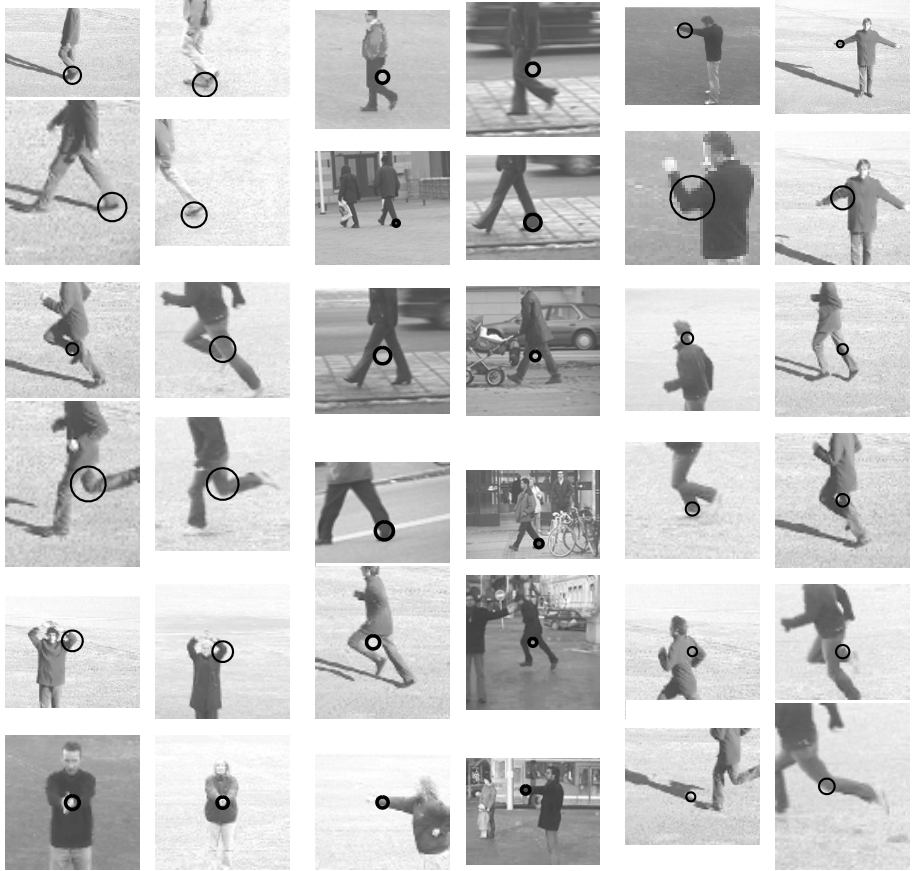
Fig. 3. Examples of point matches of space-time interest points using local image descriptors in terms of position dependent histograms of spatio-temporal gradient vectors
