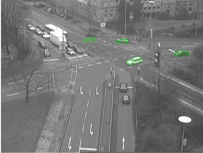
Fig. 2. Overview of the dt_passat03 image sequence at frame 953. The vehicles at the traffic light are standing and, therefore, have not been tracked yet.
