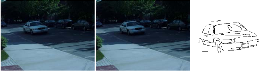
Fig. 2. The contour fragments of a moving vehicle are segregated from the background using only the two adjacent frames shown
