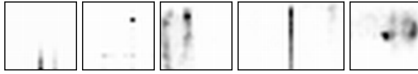
Fig. 5. The 2d space of x -motion ( x -axis) and intensity ( y -axis) of feature points from Figures 1,2,9,10 and 12 respectively. Darker means more instances of features.
