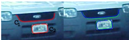
Fig. 9. Green curves in frame 2 are modeled similarity transformations of the red curves in frame 1 while blue curves are the actual curves in frame 2
