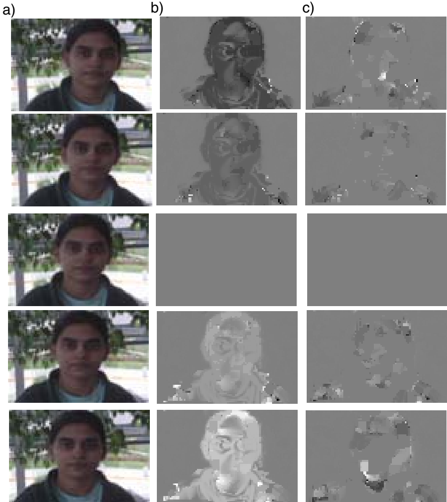
Fig. 5. a) Five (alternate) frames from the sequence, with the reference frame in the middle b) horizontal component and c) vertical component of foreground motion. Pixels for motion are scaled such that white is 9 pixels shift to right (horizontal ) or up(vertical motion), and black is 9 pixels shift in the opposite direction, with gray representing no motion. We have masked the flow fields with appropriate transparency map for the frame for clarity.
