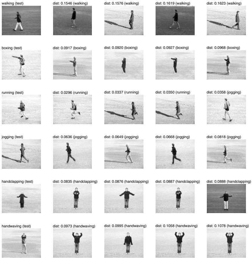
Fig. 4. One sequence for each type of action in the database [23] with its best sorted matches (ordered from left to right). Here, all matches are correct except for the sequence with “running” for which the fourth best match is “jogging”.
