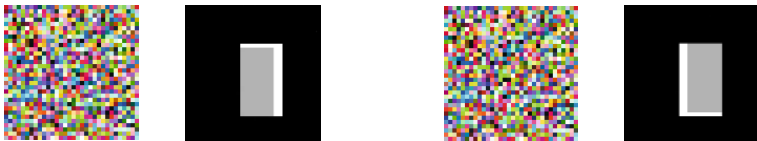
Fig. 3. Artificial flow sequence images (noisy images) generated by moving a 8 \times 16 pixel block (foreground object) by 2 pixels right and one up in front of a 32 \times 32 pixel image (containing uniformly distributed noise, pixelwise independent). Ground truth optical flow is displayed right of each image, i.e. black pixels have the same position in both images, grey ones are displaced. Pure white pixels are occluded in the other image.
