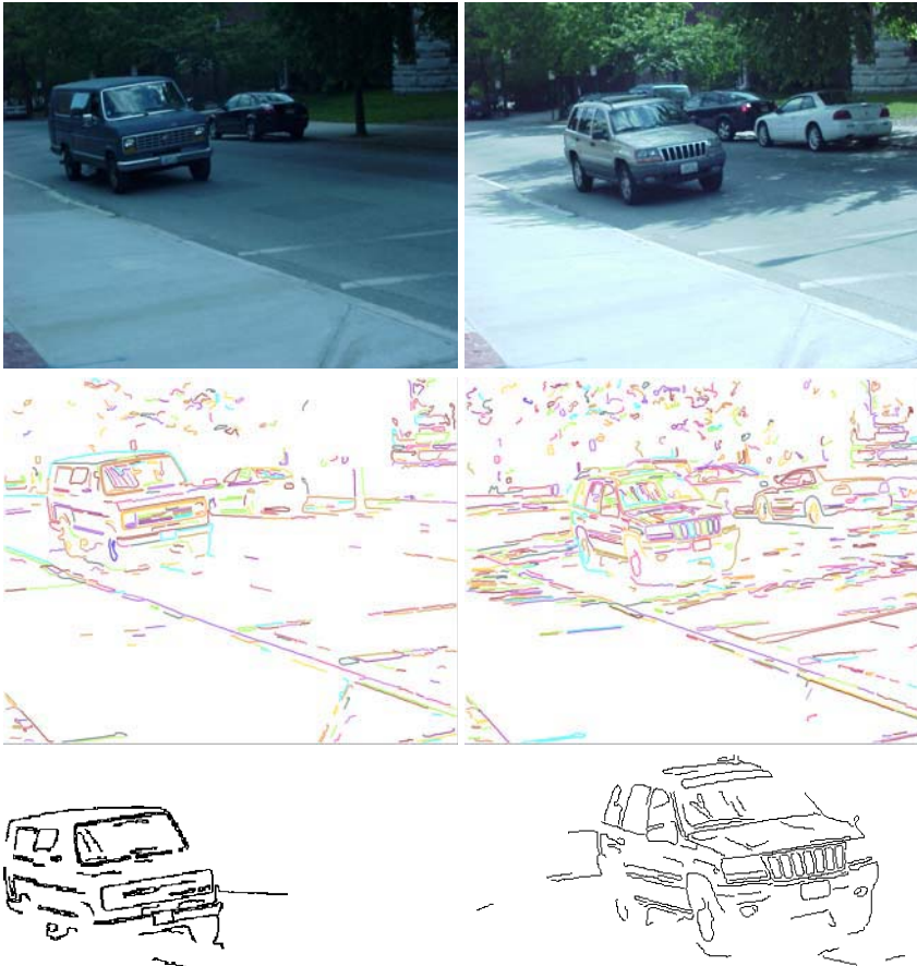
Fig. 11. Results of Figure-ground segregation based on two adjacent frames for a Van (first frame shown on the left) and an SUV (first frame shown on the right). The top row shows the original image, the second row shows the contours extracted and last row shows the segmented object.
