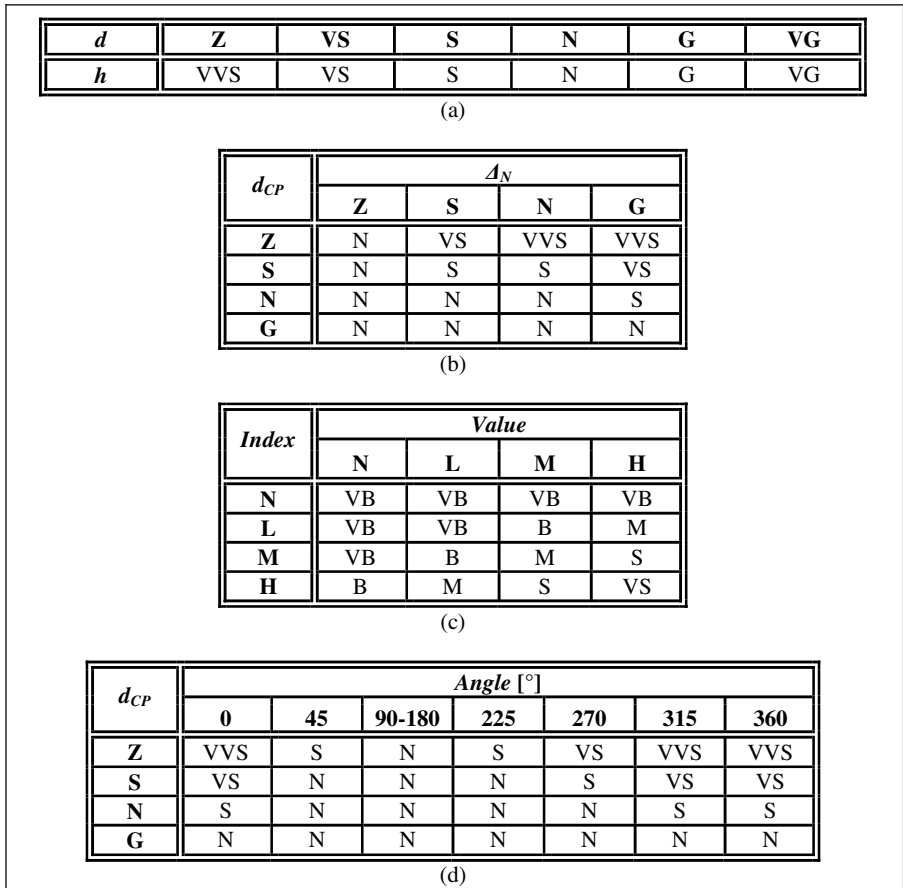
Fig. 5. The four rules sets in the table format. (a) Type Fuzzy Rules (b) Discontinuity Fuzzy Rules (c) Domain Fuzzy Rules; (d) Connectivity Fuzzy Rules. As an example, in (c) if the function in a point of the domain has a medium value and the importance of the maximum of the function is low , the dimension of the element is big .
