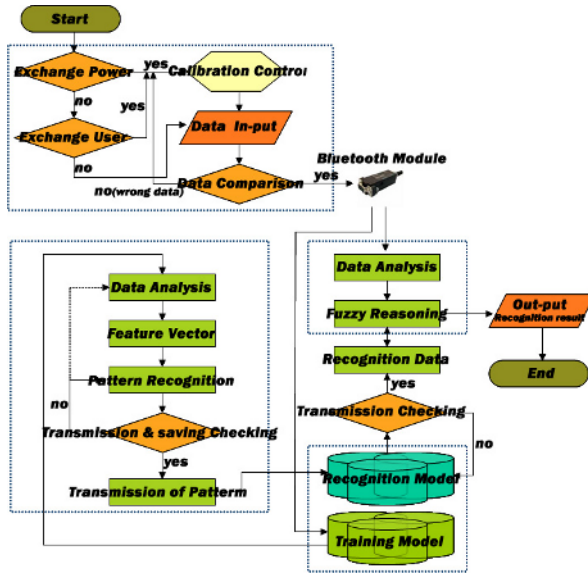
Fig. 7. The flow-chart of fuzzy gesture recognition system
