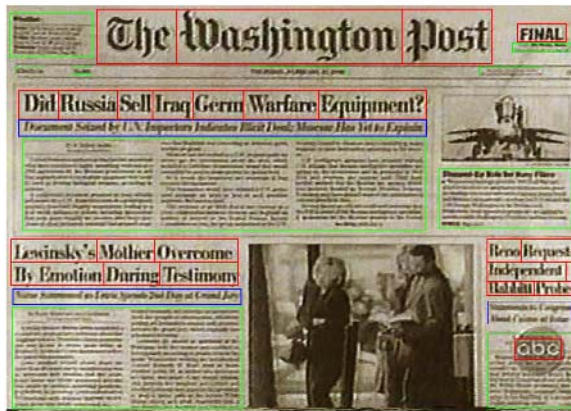
Fig. 1. Sample annotation of text in broadcast news using rectangular boxes. Textual features such as readability, size and font are used as guides for marking the edges of the box. Internally, a unique Object ID is maintained for each of the text objects shown which helps in measuring the performance of tracking. Courtesy: CNN News.
