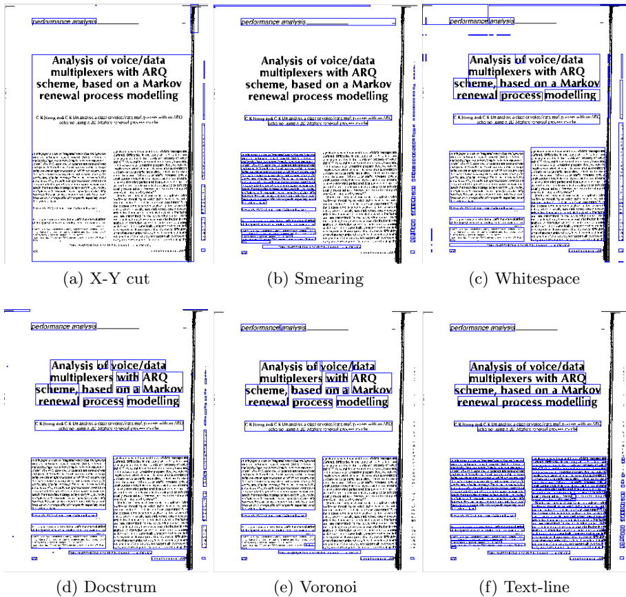
Fig. 2. Segmentation results from applying each algorithm to one page image. The page contains a title in large font and a big noise strip along the right border. (a) The X-Y cut algorithm fails in the presence of noise and tends to take the whole page as one segment. (b) The smearing algorithm also classifies the detected regions as text/non-text, and thus misses the lines joined by the noise bar. (c),(d),(e) Due to the large font size and big inter-word spacing, the Voronoi, Docstrum, and whitespace algorithms split the title lines. (f) Due to the noise bar, several characters on the right side of each line in the second column were merged with the noise bar and the text-line finding algorithm did not include these characters.
