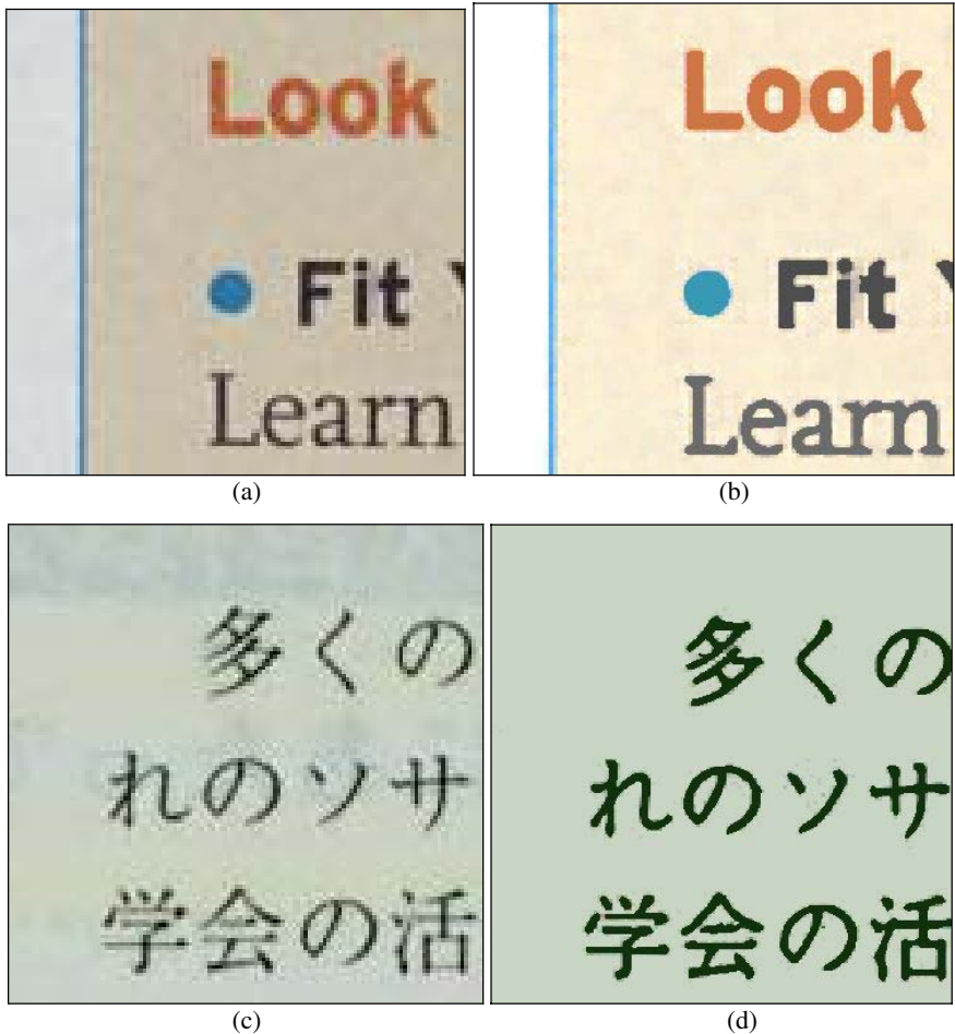
Fig. 5. Examples of optimized images for printing. (a) Normalized original image in 200dpi. (b) Optimized image. (c) Normalized original image. (d) Optimized image.
