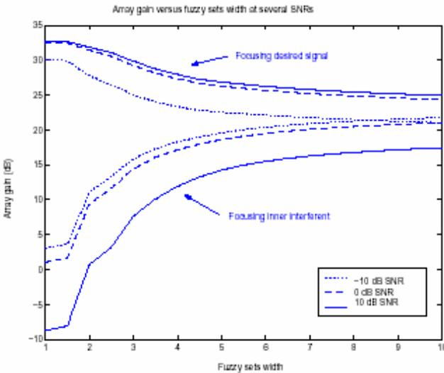
**Fig. 8.** Fuzzy beamformer array gain versus fuzzy sets width at different SNR focusing either desired or in-prior interference signal. Same scenario as Fig. 7.
