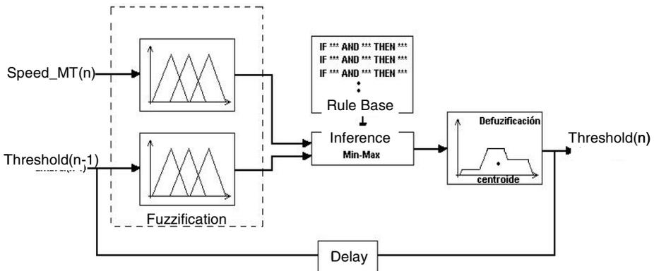
**Fig. 21.** Fuzzy controller for the hand-off threshold
