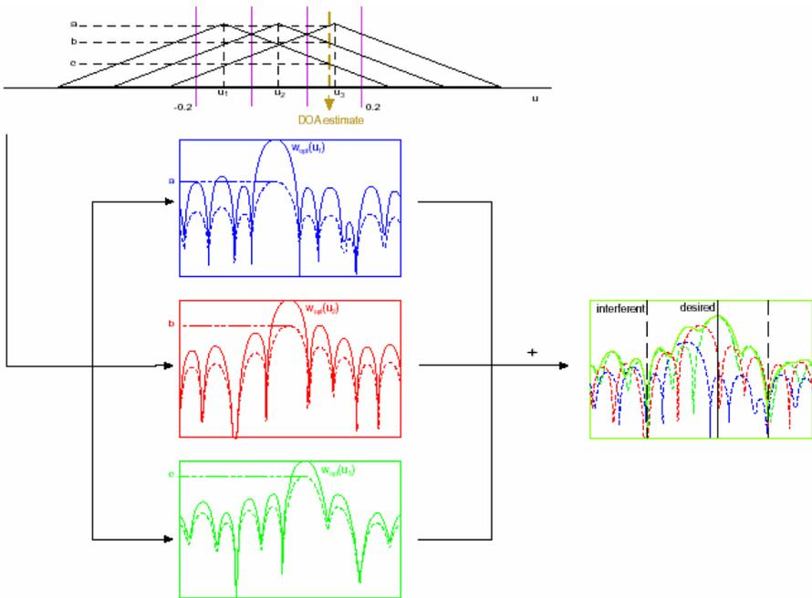
Fig. 6. Beamforming example for the case  $L=3$
