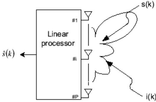
**Fig. 5.** An example of spatial linear processing to filter out a signal  $s(k)$  in presence of an interference  $i(k)$
