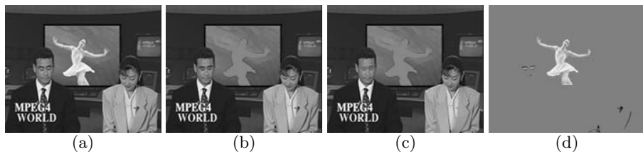
Fig. 19. Example of motion connected operator preserving fixed objects: (a) Original frame, (b) Motion connected operator \psi , (c) Dual operator: \psi^*\psi(f) and (d) residue: f - \psi^*(\psi(f))
