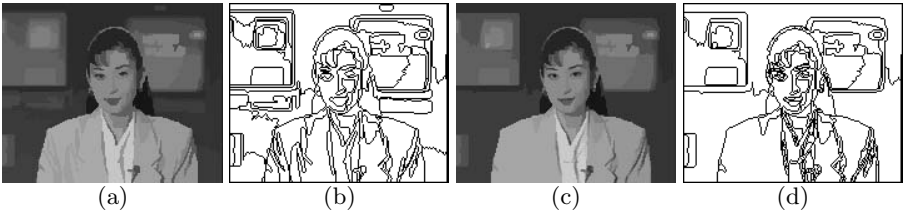
Fig. 20. Example of optimization strategies under a squared error constraint of 31 dB. (a) Minimization of the number of the flat zones, (b) contours of the flat zones of Fig. 20(a) (number of flat zones: 87, perimeter length: 4491), (c) Minimization of the total perimeter length, (d) contours of the flat zones of Fig. 20(b) (number of flat zones: 219, perimeter length: 3684).
