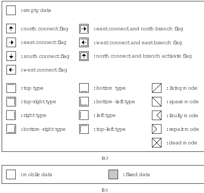
Fig. 3. The characters forming the alphabet of an artificial genome. (a) Graphical representations of the characters which are divided in 3 major classes: empty data, flag data describing the paths between the molecules of the cell, and structural data describing both the position (type) and the state (mode) of each molecule. (b) Graphical representation of the status of each character defining mobile or fixed data.
