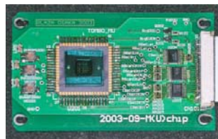
Fig. 4. Sensor module of the TOMBO system
