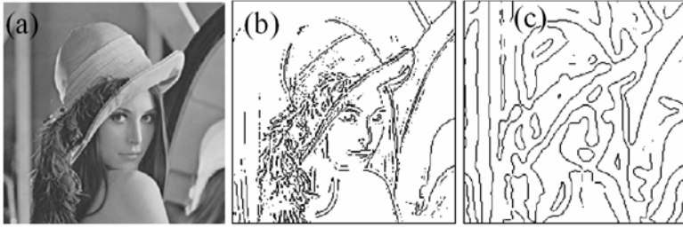
Fig. 4. (a) The famous bench-mark image of Lena. Zero-crossings detected with LOG at (b) a fine scale, the Gaussian \sigma = 1 (c) a coarse scale, the Gaussian \sigma = 4 .
