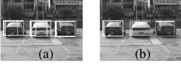
Fig. 10. Vehicle detection without and with position information of the subregions, as show in (a) and (b), respectively
