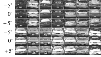
Fig. 4. Original ( 0^0 ) and synthetic canonical vehicle images ( -5^0 and +5^0 )
