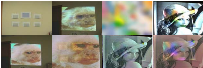
Fig. 9. Radiometric compensation. The right-top image shows that the projection color was distorted due to the texture of projection surface. There is no color distortion in the left-bottom image by compensating the projector input image. The right-bottom image shows the change of pixel values of projector input image for compensating the color distortion.
