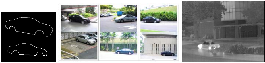
Fig. 4. (a) Edge orientation is included as additional information. (b) Some of the test images. (c) One of the infra-red images used in experiments.
