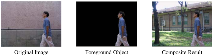
Fig. 9. The composite result. By applying the digital matting approach, we can have the composite images by replacing the background scenes in the video sequence.
