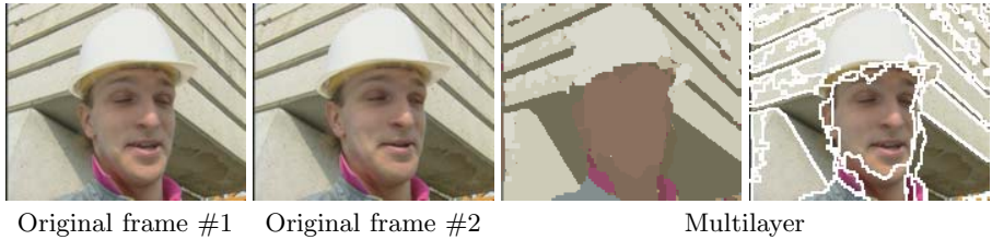
Fig. 5. Results of color only, motion only, and combined models using the motion compensated motion model . Segmented regions are shown as a cartoon image (region pixels are displayed using the average color of their region) in the first column while boundaries are overlaid on the original image in the second column of the result images.
