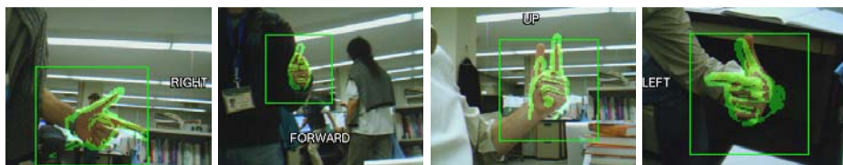
Fig. 6. Navigation by pointing at the camera. This figure shows frames from a test sequence. The overlays represent the estimated pose. Each template is labeled as one of the classes forward , left , right , up , down , stop . The examples are from four sequences where three different users perform the gestures.
