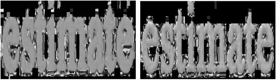
Fig. 2. Hue image of inkjet (left) and photocopied inkjet (right) print samples
