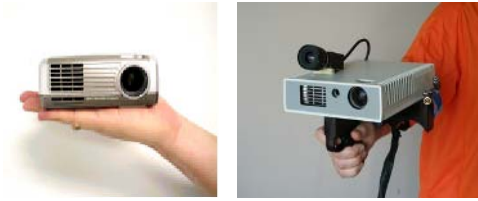
Fig. 1. At left, a commercial ‘pocket projector’; at right, our current prototype handheld projector with camera and grip
