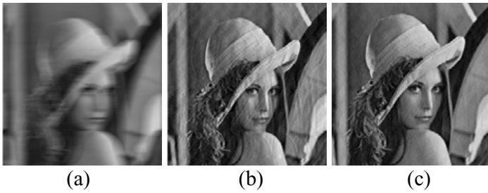
Fig. 3. (a) Blurred noisy image, 512 \times 512 pixel. (b) Restored image based on Lucy-Richardson algorithm 100 iterations with known PSF, ISNR=5.35 dB. (c) Blind image deconvolution using our algorithm, ISNR = 6.16 dB.
