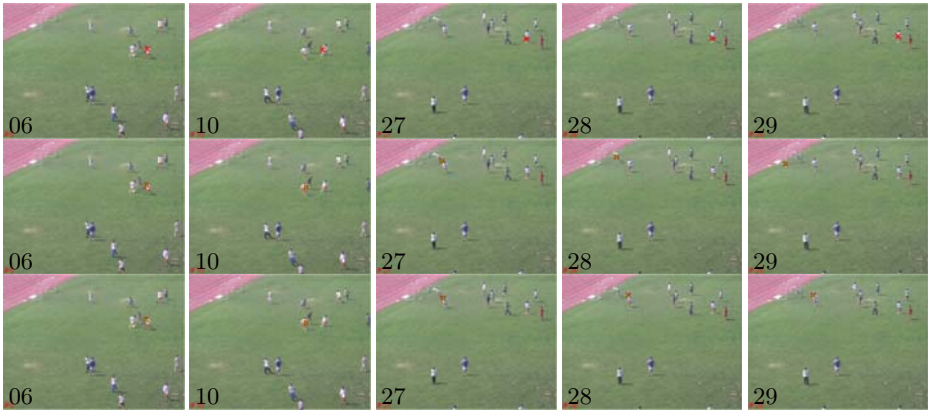
Fig. 3. In these tracking result sequences, player position estimated is marked with a red cross. The first row displays mean shift only tracking result. The second row shows the result of Kalman + mean shift method. And the result of our method, pseudo measurement based multiple model approach, is put in the third row.
