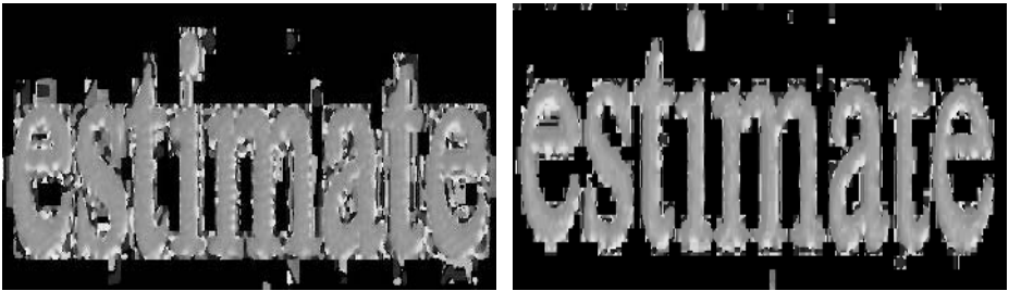
Fig. 3. Hue image of laser (left) and photocopied laser (right) print samples
