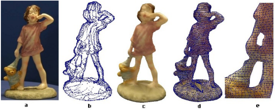
Fig. 3. Reconstruction of a girl and teddy toy with complex topology from a turntable sequence (20 images). (a) The original image. (b) Recovered 3D rims. (c) Resulting surface with texture mapping. (d) Resulting surface with the wire-framed mesh superimposed. (e) Local view of the mesh.
