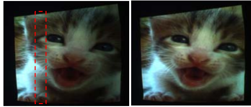
Fig. 10. Intensity-compensated projection. Left image: a projector lights the cylindrical surface on the left side and thus the left part of the image is brighter than the right part of the image. Right image: after compensation, the brightness of the whole image became similar.
