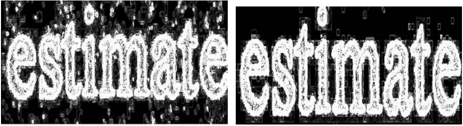
Fig. 6. Edge-detected hue image of inkjet (left) and photocopied inkjet (right) samples
