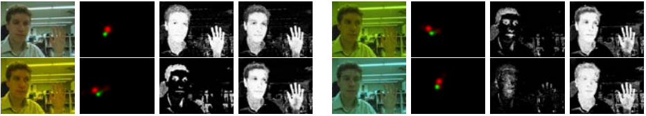
Fig. 2. Colour adaptation based on face detection. Each of the four examples shows the input frame from a sequence with varying colour balance, the smoothed skin colour (green) and background distributions (red) in UV-colour space, probabilities for a static colour model in normalized UV-space, probabilities for the adaptive model based on face detection.
