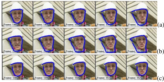
Fig. 1. Predictor comparison I: (a) The tracking results by using the affine predictor for frames 148-152. The previous 2 frames are used to predict the affine matrix. (b) The tracking results by using the affine predictor for frames 148-152. The previous 4 frames are used to predict the affine matrix. (c) The tracking results by using the proposed shape prediction matrix for frames 148-152. The total number of frames used for estimating the shape prediction matrix is 40.
