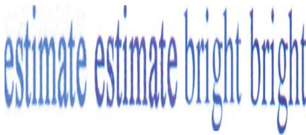
Fig. 1. Samples of inkjet printing, its photocopy, laser printing and its photocopy
