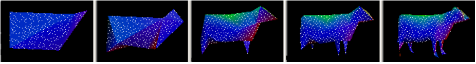
Fig. 1. 3D models level-of-detail. The leftmost model has the least number of polygons. White points on the model are data samples. The models are shaded according to surface normal profiles on the polygonal surfaces.
