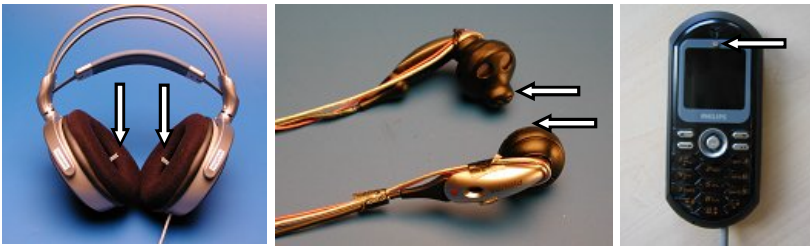
Fig. 4. The three platforms: headphones, earphones and mobile phone all with extra microphones indicated by arrows
