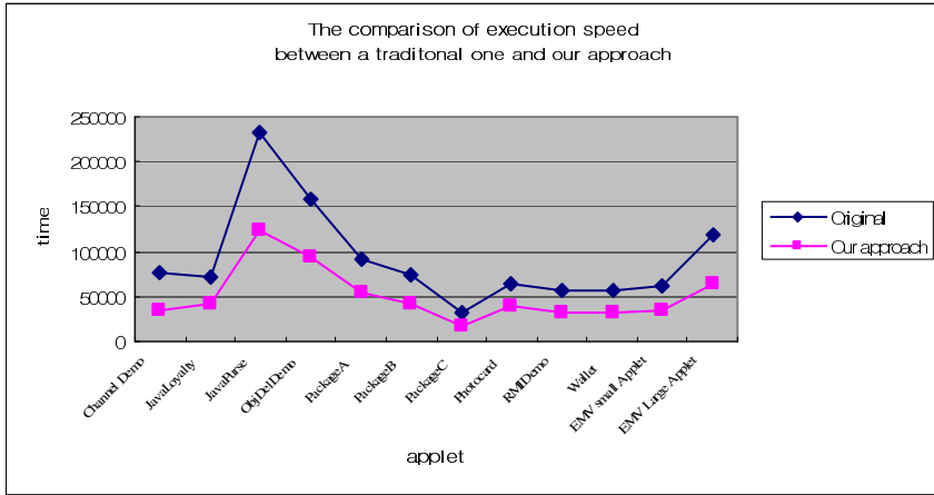
Fig. 14. The comparison between a traditional Java Card and our changed Java Card with regard to an execution speed
