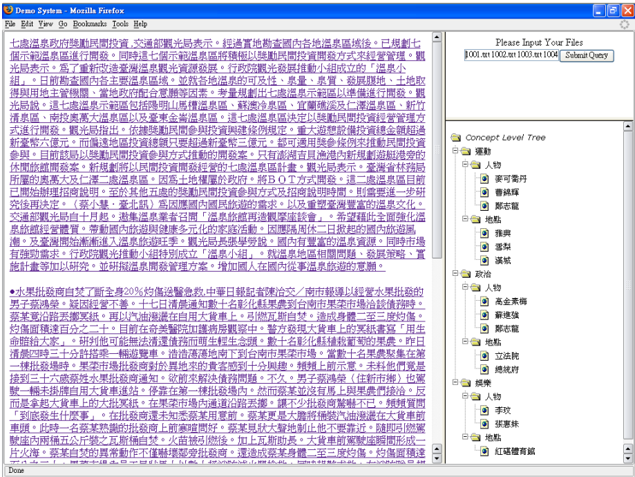
Fig. 2. A prototype information summarization system allowing users to browse documents with the categorized key terms and user-defined categories
