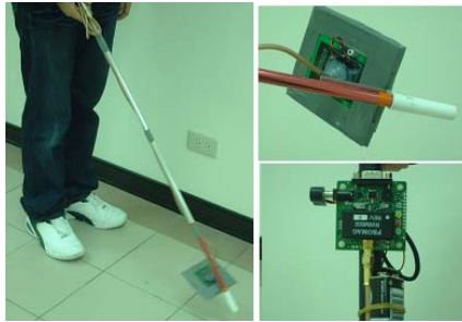
Fig. 2. On the left hand side of the figure is the iCane overview; on the top right of the figure is our RFID antenna; on the bottom right of the figure is our RFID reader
