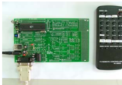
Fig. 6. The IR receiver and the remote controller
