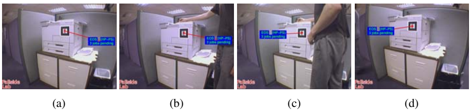
Fig. 4. Example of the dynamic behaviour. (a) A label is placed in an uninteresting position. As a person moves into the view (b), the label jumps to another location (c). The weak position prior prevents the label from quickly jumping back to the previous position (d).
