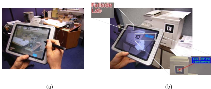
Fig. 1. A hand-held augmented reality system for information browsing using labels attached to markers and “screen-stabilized” labels. The system determines the label locations in real-time in such a way that overlap with interesting parts of the image is minimised.
