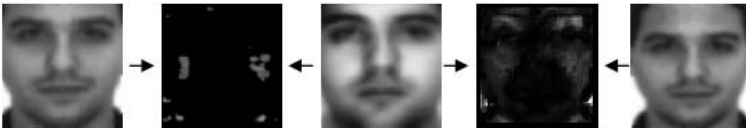
Fig. 3. Illustration of the effect of misalignment of test image with the face model in the center
