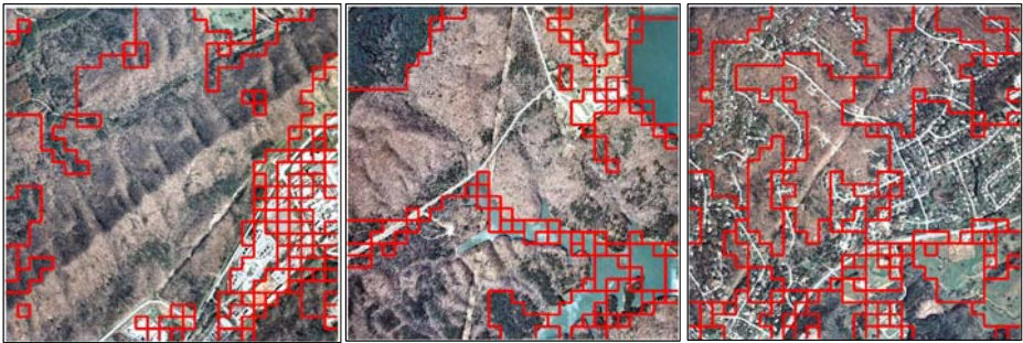
Fig. 8. Region growing results across three tiles from the image library. Each bordered region represents one homogeneous, connected group of segments as determined by their texture and structure features.
