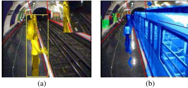
Fig. 7. Limitations of the current implementation of the system. (a) Small object thrown on the tracks; (b) illumination variations generated by the train on the platform.
