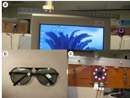
Fig. 1. Hardware setup: (a) camera setup on the computer, (b) eye-glasses with IR reflective markers, (c) camera close-up with IR LEDs
