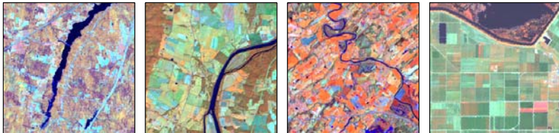
Fig. 5. Examples from the Landsat Thematic Mapper showing variation in spectral response across large geospatial extents. Three of six spectral bands have been selected for display that emphasize variations in crop cover. From left to right, Maine, Virginia, Tennessee, Florida.
