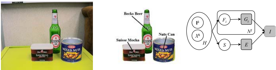
Fig. 1. Left: A simple scene with three objects ( Nuts Can , Suisse Mocha Box , and Becks Beer ) on a table. Middle: The segmentation and recognition results from our proposed algorithm. Right: Graphical representation of the proposed Bayesian belief network. The shaded box nodes denote the evidences. The circles denote the hidden variables. The ellipse denotes the hypernode composed of hidden variables. The big plate around F_i and G_i comprises N^I number of i.i.d. F_i and i.i.d. G_i .
