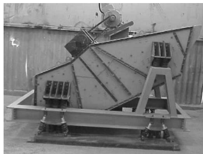
Fig. 1. Prototype on scale of a vibrating screen, used to test the intelligent control system
