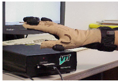
Fig. 3. The Flock of Birds® 3-D motion tracker
