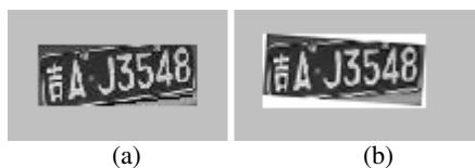
Fig. 6. (a) Angle detecting using Radon transform. (b) Rotated result according to the angle.
