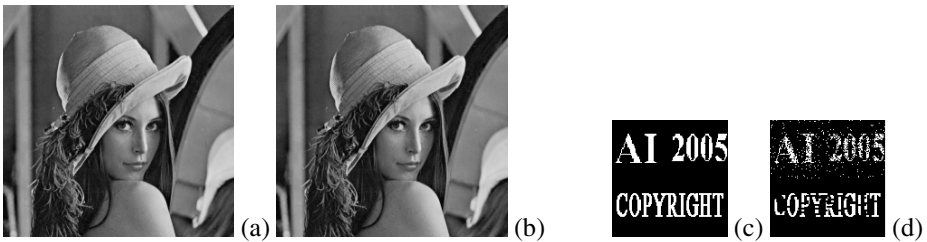
Fig. 2. (a) Original host image ‘Lena’. (b) Watermarked result image. (c) Extracted watermark from Fig. 2(b). (d) Extracted watermark from Fig. 2(b) after cropping attack.
