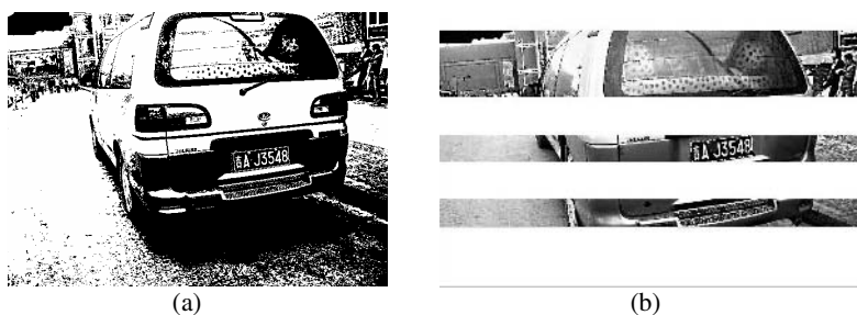
Fig. 3. (a) The binary image. (b) Three candidate zones extracted from grayscale image.
