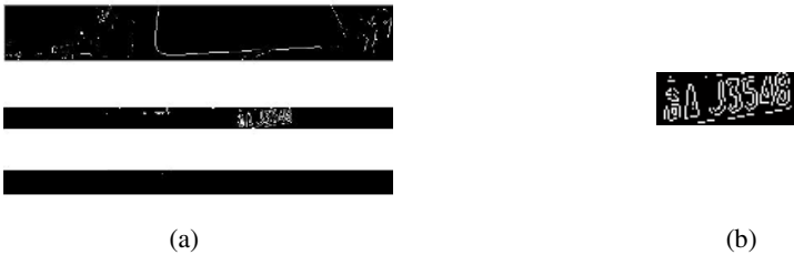
Fig. 4. (a) The results of edge detection for three candidate zones. (b) The real license plate detecting using Vertical-cutting algorithm.
