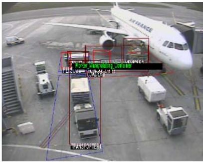
Fig. 3. (Left) Two dynamic zones (in blue) linked with the Loader and the Transporter vehicles involved in the event “Worker_Manipulating_Container” (event 26) detected. (Right) The Unloading operation involving 8 physical objects and 3 composite components with 2 constraints on the vehicle subtypes, 4 constraints on the zones of interest and 2 temporal constraints.
