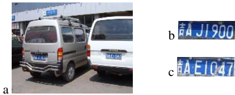
Fig. 1. (a) Original image. (b) The license plate region 1. (c) The license plate region 2.
