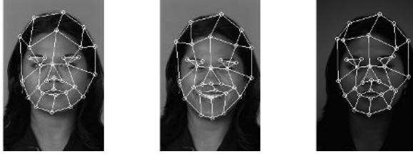
Fig. 4. Face images belonged to the same person with normal expression ( fa and ba image), smiling expression ( fb and bj image) and under darker illumination ( bk image). The graphs in the images were generated automatically utilizing DE algorithm and FBG structure.
