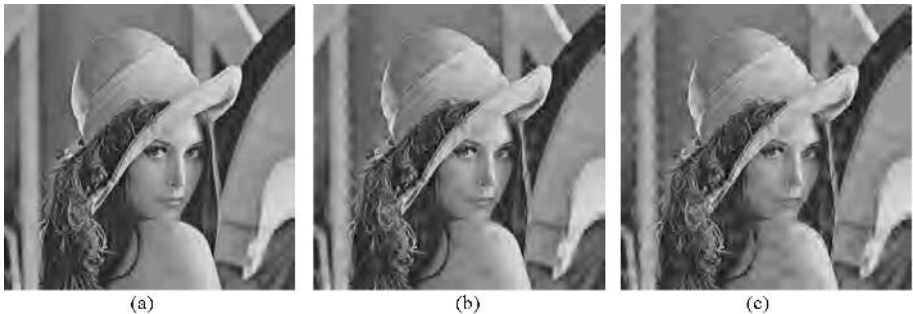
Fig. 8. Reconstruction "Lena" at 0.1bpp by TMDC1 : (a) with all descriptions; (b) with 2 row descriptions (4-5) lost; (c) with 4 row descriptions (3-6) lost
