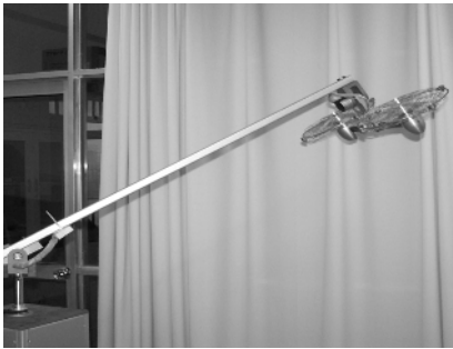
Fig. 2. Tilt rotor aircraft platform experimental setup Fig. 3. Tilt rotor aircraft platform scheme
