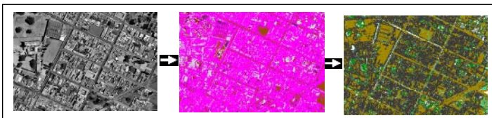
Fig. 6. Airplane image and the CLS recognition: Level 3 land segment Land 4 urban segment
