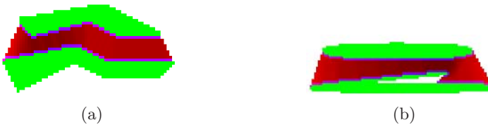
Fig. 2. (a) Region between two objects, calculated by the visibility approach; (b) Analogous to (a), but showing that the concavity of one of the objects is properly excluded from the between region by the visibility method.
