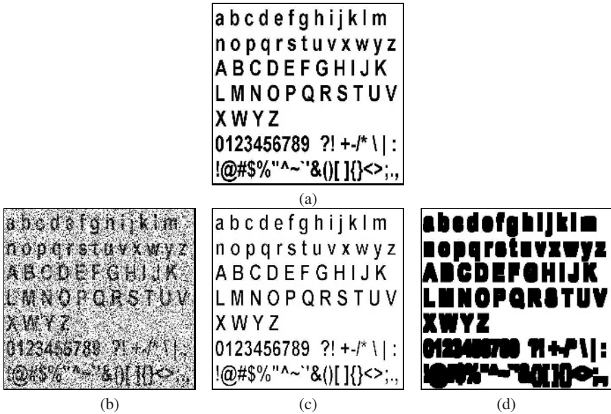
Fig. 1. Test images: (a) Ground-truth image, (b) Salt-Pepper (50%), (c) Dilation (cross EE 1 iteration), (d) Erosion (square EE 5 iterations)
