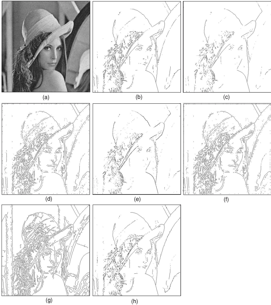
Fig. 4. (a) Original image 10 percent contaminated, standard deviation 80. Edge detection methods:(b) Prewitt (c) Sobel (d) Log (Laplacian of normal) (e) Roberts (f) Zero-cross (g) Canny (h) Proposed.
