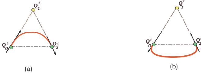
Fig. 5. Interpolating the sense of tangent vectors. (a) Inner case (b) Outer case .
