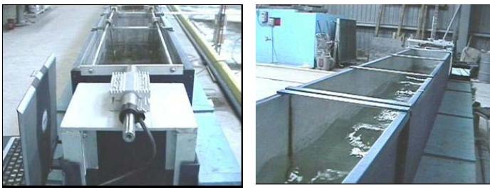
Fig. 2. Linear motor with paddle device and a channel of irregular and unidirectional wave
