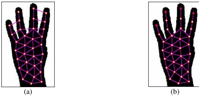
Fig. 4. (a) Hand image after the application of the SGONG network, (b) hand image after the location of the raised fingers
