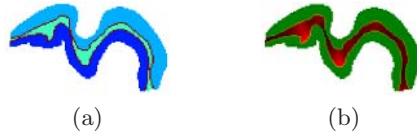
Fig. 3. Results using the visibility approach to calculate \beta . (a) Synthetic shapes and the region \beta between them. The adjacent arcs are also indicated. (b) The distance map D_{AB}(x) in \beta is represented as grey-levels.
