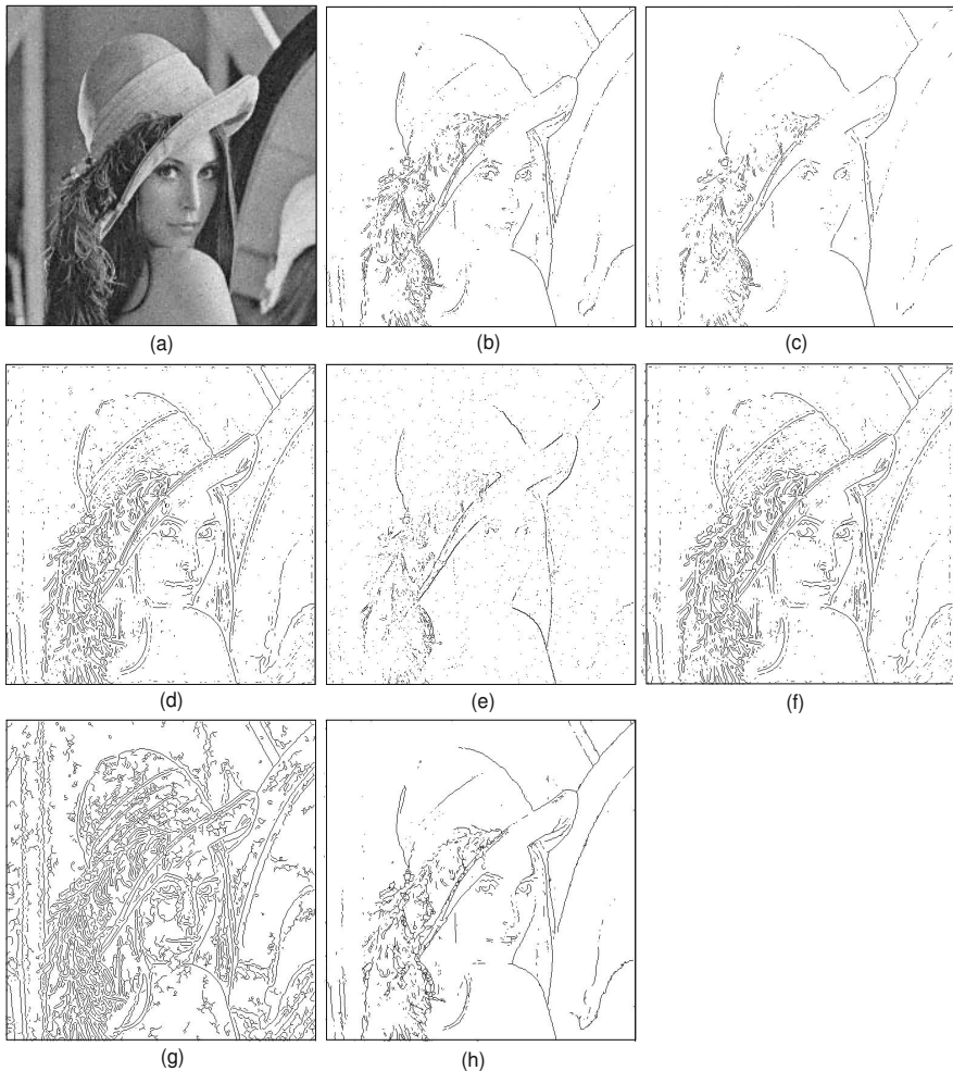
Fig. 3. (a) Original image 25 percent contaminated, standard deviation 40. Edge detection methods: (b) Prewitt (c) Sobel (d) Log (Laplacian of normal) (e) Roberts (f) Zero-cross (g) Canny (h) Proposed.
