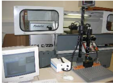
Fig. 1. The camera and the lighting system
