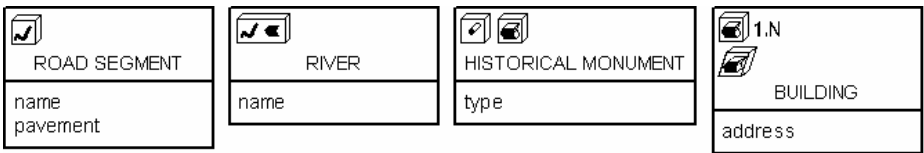
Fig. 2. Examples of PVL grammar rules in UML classes for objects respectively having simple, complex, alternate and multiple geometries (the latter including 2 geometries, one of them being a multipolygon aggregate)
