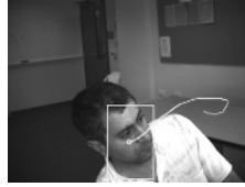
Fig. 1. Face tracking using mean-shift algorithm and boundary density thresholding method
