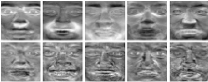
Fig. 3. Visual representation of the lower components (or base vectors) of PCA (top row) and EFM (bottom row) of the face, respectively
