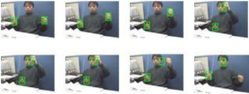
Fig. 3. Tracking failure by color and motion based Mean Shift algorithm
