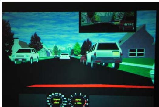
Fig. 1. STISIM simulator driving software showing front and rear views together with speedometer and rev counter
