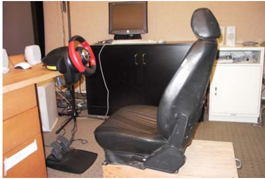
Fig. 2. Simulator driving hardware including pedals for an automatic car, steering wheel and car seat
