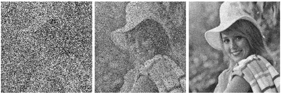
Fig. 6. (Example 2) The true image with 75% salt-and-pepper noise, 50% random-valued impulse noise and additive Gaussian noise ( \sigma = 20 ) respectively
