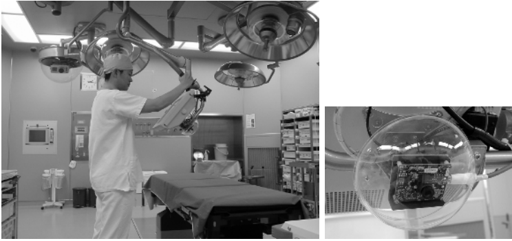
Fig. 3. The setup of a data-fusion display. The operator is grabbing and moving the monitor to the position from where he wants to observe the inner structure. A small video camera is inset in the backside of the monitor.
