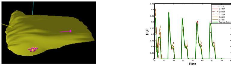
Fig. 4. (a) 12 vertices (pink dots) which have the lowest df with a sample vertex (yellow dot) (b) overlapping HVS curves of these vertices (Green curve is the distribution of sample vertex).
