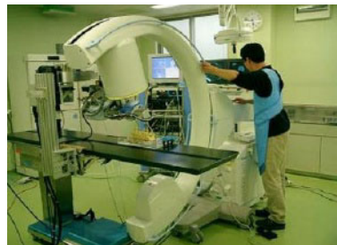
Fig. 7. The robot can be installed between a patient and C-Arm X-Ray Equipment
