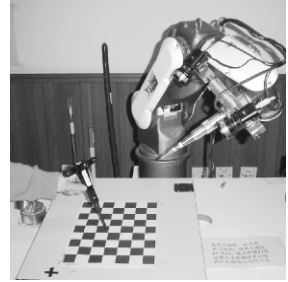
Fig. 4. Positioning test with the infrared probe
