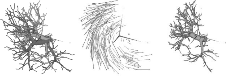
Fig. 1. [Left] A large deformation case is pruned at 20% (% of branch area randomly removed in both trees). [Center] The figure shows the result of our oriented tree matching, good matches are represented by light gray arrows and represent 91% of all nodes and wrong matches by dark gray arrows. [Right] The figure shows the tree registration after the process.
