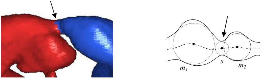
Fig. 1. Left: A narrowing and a possible cut. Right: Medial Axis (dashed line) of a two dimensional object (interior of the solid lines) and two locally maximal medial balls m_1 , m_2 and the smallest medial ball s between m_1 and m_2 . The ball s lies at the narrowing between m_1 and m_2 .
