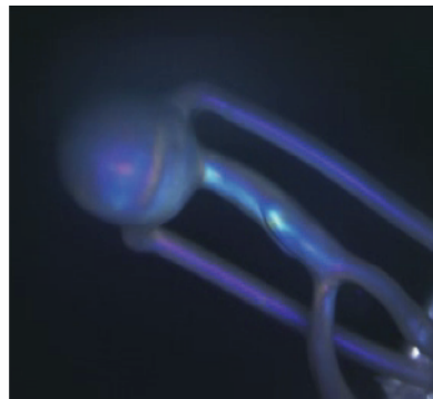
Fig. 6. Stress distribution against catheter operation visualized by means of photoelastic effect with reflective circular polariscope
