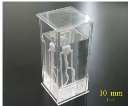
Fig. 4. Cerebral arterial model with vascular-like membranous configuration and brain-like soft circumferential configuration
