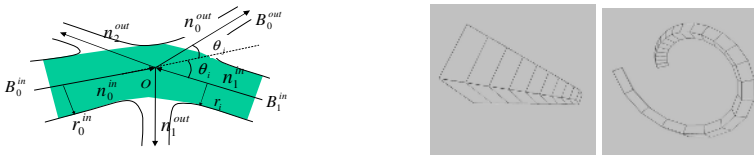
Fig. 1. Left: Trunk branch selection: using both vessel average radii and branching angle to determine the continuation trunk branch. Although \theta_j < \theta_i , B_1^in is chosen as the trunk branch of B_0^in , due to the similarity of their average radii. Middle: Cross section distribution gets denser at thinner regions of a vessel. Right: the density is higher where a vessel turns or twists.
