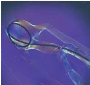
Fig. 5. Stress distribution against catheter operation visualized by means of photoelastic effect with circular polariscope
