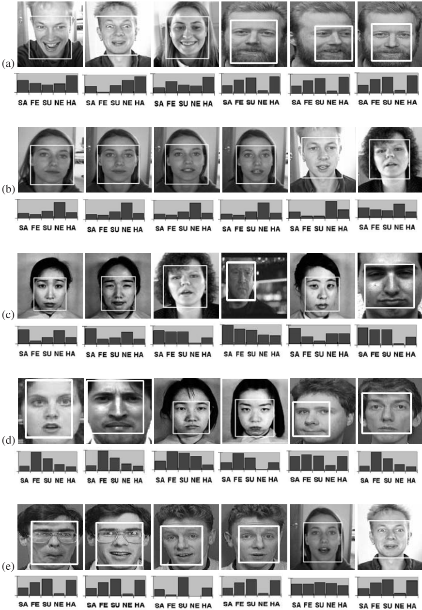
Fig. 5. Performance on several test images — (a) happy (b) no expression (c) sad (d) fear (e) surprise. For each test image, the corresponding graph below shows the probability of each of the five expressions.
