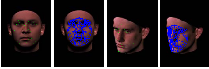
Fig. 5. Building dense correspondence between the rotated view and the frontal view using sparse features. The first and second image show the sparse features and the constructed meshes on the mean face at the frontal pose. The third and fourth image show the picked features and the constructed meshes on the given testing image at the rotated pose.
