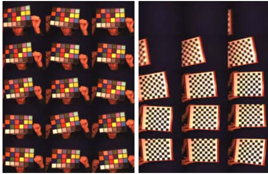
Fig. 8. Sample images of color (left) and camera (right) calibration data. Here we show 15 intermittent frames for the front camera.
