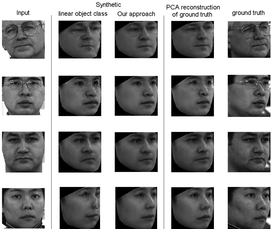
Fig. 5. Synthesizing a 45^\circ view from a given frontal view. Column 1 to 5: (1) input image under pose 1 (2) synthetic image using linear-object-class. (3) synthetic image using our approach. (4) PCA reconstruction of ground truth of pose 2. (5) ground truth of pose 2.
