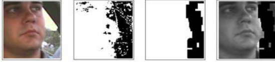
Fig. 7. An example of the face pixel segmentation result. First image: detected face; Second image: segmented face pixels (white color: face pixels); Third image: refined face pixel mask; Fourth image: segmented face pixels.
