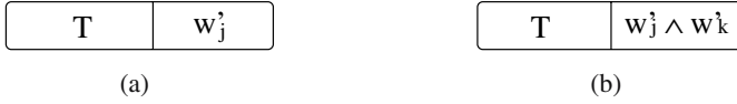
Fig. 2. (a) P_i sends P_j a BDD message with an assumed window w'_j (b) P_j forwards a BDD message to P_k with an assumed window w'_k
