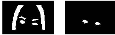
Fig. 4. Eye candidate regions extracted template matching and the eye region picked out from the candidates using location information on the eyes ( left and right )
