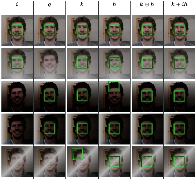
Fig. 2. Face detection examples under some of the artificial brightness distortions from our first series of experiments. Combined curvature features are most reliable in the case shown here.
