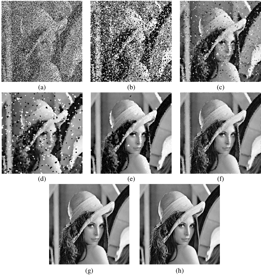
Fig. 4. Restoration results of different median-based filters. (a) Corrupted image “Lena” with 60% salt-and-pepper noise. (b) Median filter with 3 \times 3 window size. (c) CWM filter with 5 \times 5 window size and a center weight of 3. (d) IM filter with 3 \times 3 window and 10 iterations. (e) PSM Filter. (f) AM filter. (g) Proposed NASM filter. (h) Original test image of “Lena”.
