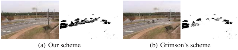
Fig. 2. Background image and object segmentation at time 3841 with learning rate \alpha = 1/1024
