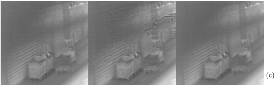
Fig. 2. Performance of the NUC methods under real IR data. (a)(b)(c) The 1611 - th ( 1134 - th ) ( 1340 - th ) frames of the first (second)(second) set of IR data, at the left the raw frames, at the center the corresponding frames corrected by our previous enhancement to Scribner's NUC method and at the right are the frames corrected by proposed method.
