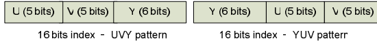
Fig. 3. 16 bits index for color space transformation lookup table. (UVY pattern V.S. YUV pattern) The former encounters more cache hits.
