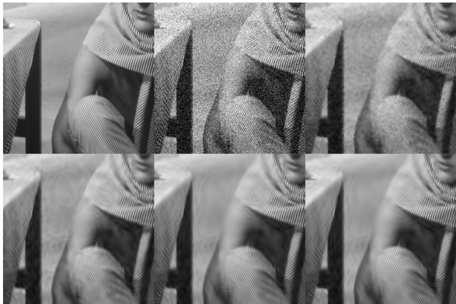
Fig. 2. Cropped images ( 256 \times 256 ) using proposed algorithms for 512 \times 512 Barbara image with \sigma=30 : Original (top-left), Noisy (top-center; 18.58dB), Wiener filter (top-right; 24.73dB), Method 2 (bottom-left; 27.35dB), Method 1 (bottom-center; 27.92dB), Method 3 (bottom-right; 27.96dB)
