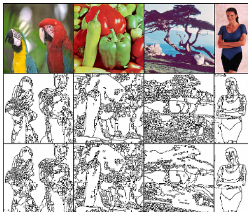
Fig. 4. Contour maps of the localization scale (initial segmentation). First row: test images Parrots, Tree and Woman. Second Row: Selected scale using LSS. Third Row: SODM results.
