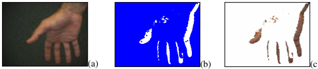
Fig. 5. A moving hand: (a) Original image, (b) In-motion pixels of the frame, filtered using Hue threshold (c) Mapping the result to the original image
