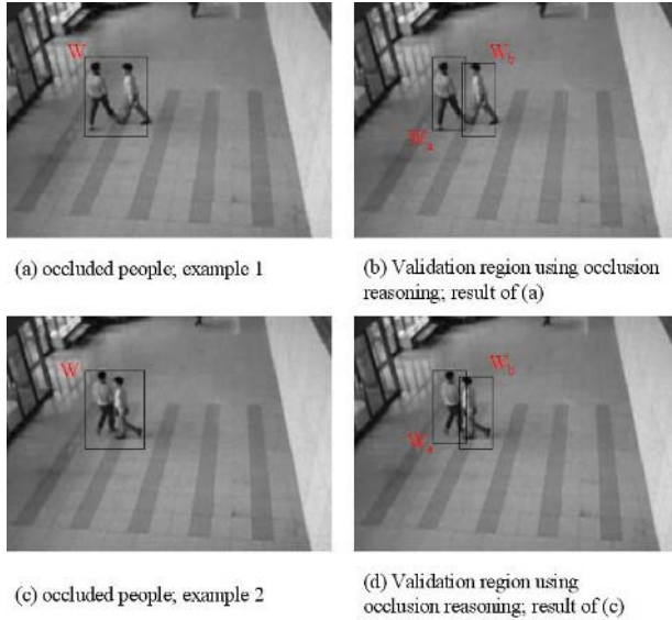
Fig. 2. Validation region using occlusion reasoning
