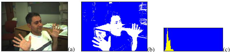
Fig. 1. (a) Original Image, (b) Filtered image based on thresholding Hue factor of skin color extracted from training data, (c) Hue histogram of the training data
