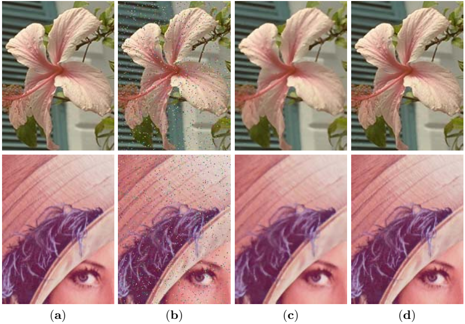
Fig. 7. Illustrative examples of the filtering efficiency: a) zoomed parts of the color test images, b) images contaminated by 5% uniform noise, c) restoration achieved with the VMF, d) filtering results achieved using the new noise detection technique
