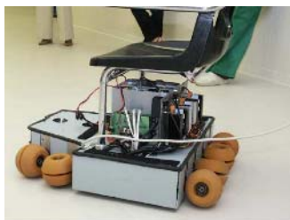
Fig. 1. Wheelchair with omni-directional wheels that inspires the developing of the platform
