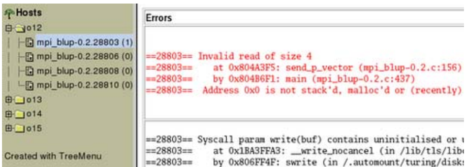
Fig. 2. The ClusterGrind HTML report - cluster nodes are represented as elements in a tree menu
