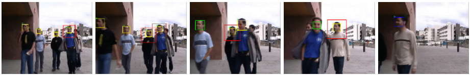
Fig. 3. Frames extracted from a video stream with 720 \times 576 resolution. The color has the same meaning than in Figure 1, but observe that the last frame depicts a blue rectangle which means that tracking was used.
