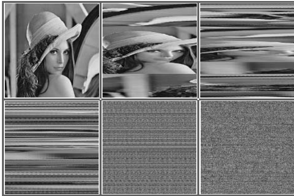
Fig. 1. Illustrating the chaotic and mixing dynamics associated when iterating a Kolmogorov system
