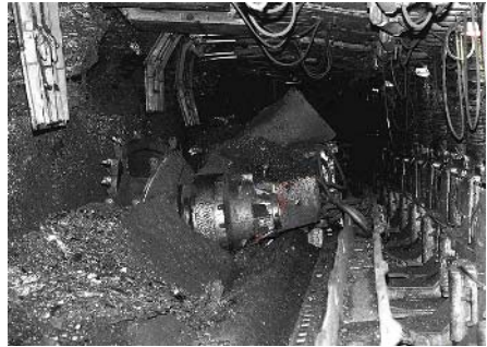
Fig. 1. Shield Supporting system and the Coal-winning shearer working
