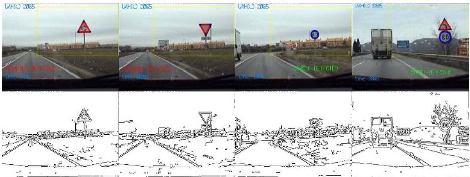
Fig. 1. Real images sequence, detected on the road, with the search area within each image outlined (square window), and Canny image used for contour-information search
