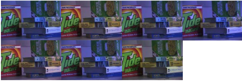
Fig. 2. Comparison to Color Constancy algorithms (Detergent image). Upper-row from left to right: original image (to be color-corrected), target image (image under canonical illuminant), GW, Retinex; Lower-row from left to right: NN, GM, IGA-GM.
