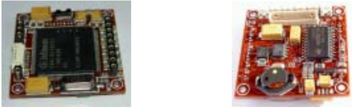
Fig. 4. The motor controller board (left: upper side, right: lower side)
